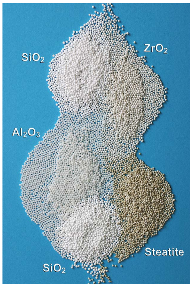
Fig. 2. Different commercial catalyst supports usable for catalyst screening with the single-bead approach.
